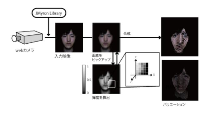
System in which image is input from web camera and is output as Pseudo Stereoscopic deformed image.
